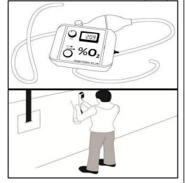
10.9.3. When carrying out a CO<sub>2</sub> treatment, the approximate CO<sub>2</sub> concentrations can be determined by measuring O<sub>2</sub> concentrations using the conversion table below:
