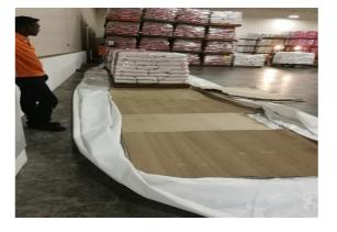
b. Cover the G-HF Cocoon<sup>™</sup> material with cartons or equivalent, and then stack the first layer lengthwise with the forklift.
