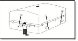
10.5.3. Use a vacuum pump [at least 2.3 cubic meters per minute with 600 Watts (0.80 horsepower) centrifugal pump]:
